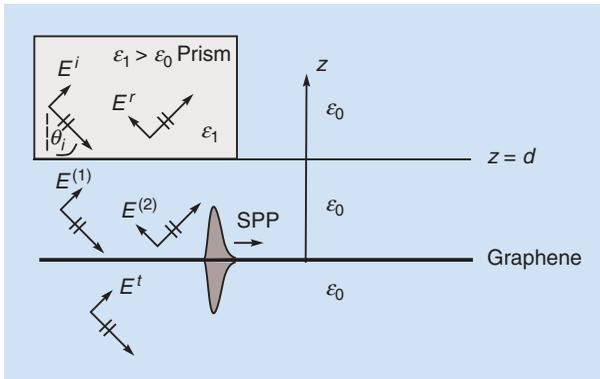
**FIGURE 3.** An incident field inside a prism coupling to quantized SPPs supported by graphene.
