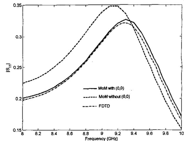
Figure 5. The return loss ( $S_{11}$ ) as a function of frequency for a longitudinal-slot waveguide radiator with the following dimensions: the waveguide was 2.286 cm  $\times$  1.016 cm, the slot was 1.6 cm  $\times$  1 mm, the slot centerline was at 0.343 cm from the narrow wall, and the wall thickness was 1.27 mm.
