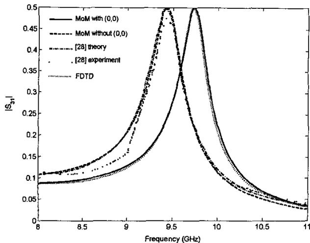
Figure 4. The coupling coefficient ( $S_{31}$ ) as a function of frequency for a longitudinal-slot waveguide coupler with the following dimensions: the waveguide was 2.286 cm  $\times$  1.016 cm, the slot was 1.56 cm  $\times$  1 mm, the slot centerline was at 0.643 cm from the narrow wall, and the wall thickness was 1.27 mm.
