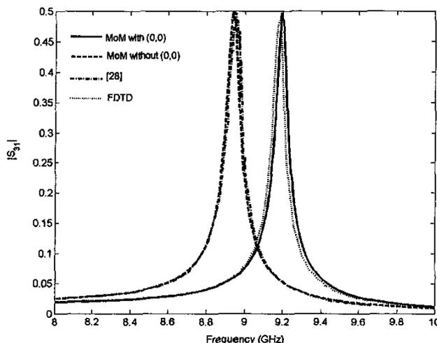
Figure 3. The coupling coefficient ( $S_{31}$ ) as a function of frequency for a longitudinal-slot waveguide coupler with a wall thickness of 2 mm.
