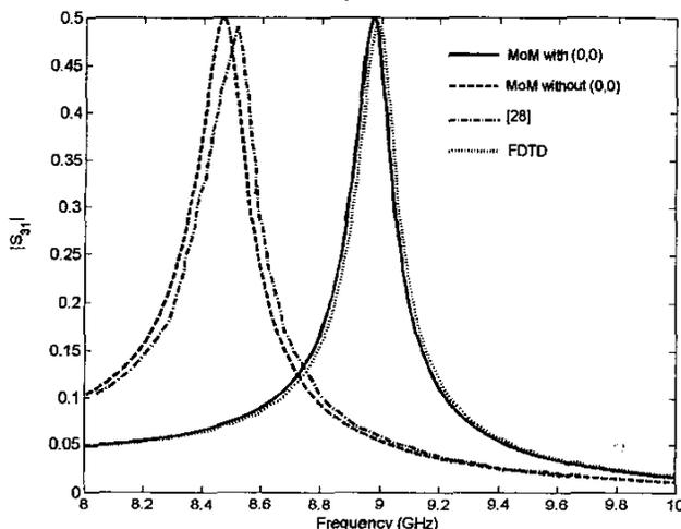
Figure 2. The coupling coefficient ( $S_{31}$ ) as a function of frequency for a longitudinal-slot waveguide coupler with the following dimensions: the waveguide was 2.286 cm  $\times$  1.016 cm, the slot was 1.6 cm  $\times$  1 mm, the slot centerline was at 0.943 cm from the narrow wall, and the wall thickness was 0 mm.
