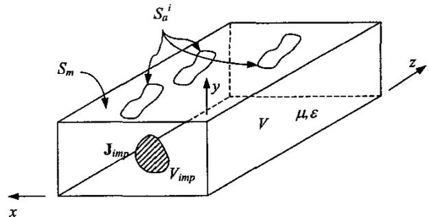
Figure 1. An infinite rectangular waveguide with arbitrarily shaped radiating slots.
