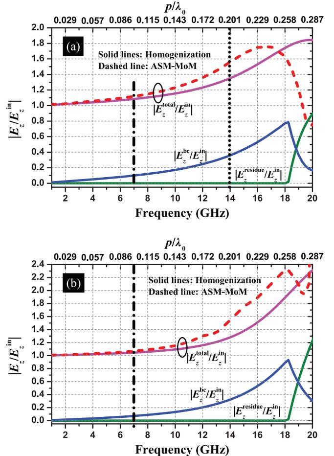
Fig. 9. Normalized total, residue, and bc  $E_z$  excited by VED source above a JC array. Structural parameters:  $p = 4.3$  mm,  $g = 0.1$  mm,  $d = 2.8$  mm,  $w = t = 0.2$  mm,  $x' = y' = 0$ ,  $x = y = \lambda_0/\sqrt{2}$ . (a)  $z' = z = \lambda_0/5$  and (b)  $z' = z = \lambda_0/10$ .
