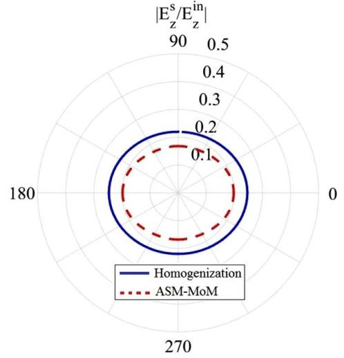
Fig. 12. Normalized scattered electric field excited by a VED source at  $f = 10$  GHz versus angle  $\phi$  for  $\rho = 0.2\lambda$  for PEC strips having width  $w = 3$  mm, period  $p_x = 3.5$  mm ( $p_x/\lambda = 0.117$ ) and height  $z = z' = \lambda/5$  ( $z/p_x = z'/p_x = 1.713$ ). Solid blue line shows homogenized results and dashed red line shows ASM results.
