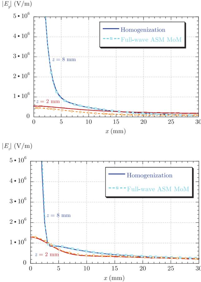
Fig. 8. Electric field excited by a 1-Amp HED (upper plot) or VED (lower plot) source above a JC array at  $f = 10$  GHz, for  $p = 4.3$  mm,  $g = 0.1$  mm,  $d = 2.8$  mm,  $w = t = 0.2$  mm,  $x' = 0$ ,  $y' = 0$ ,  $z' = 10$  mm, and  $y = 0$ .
