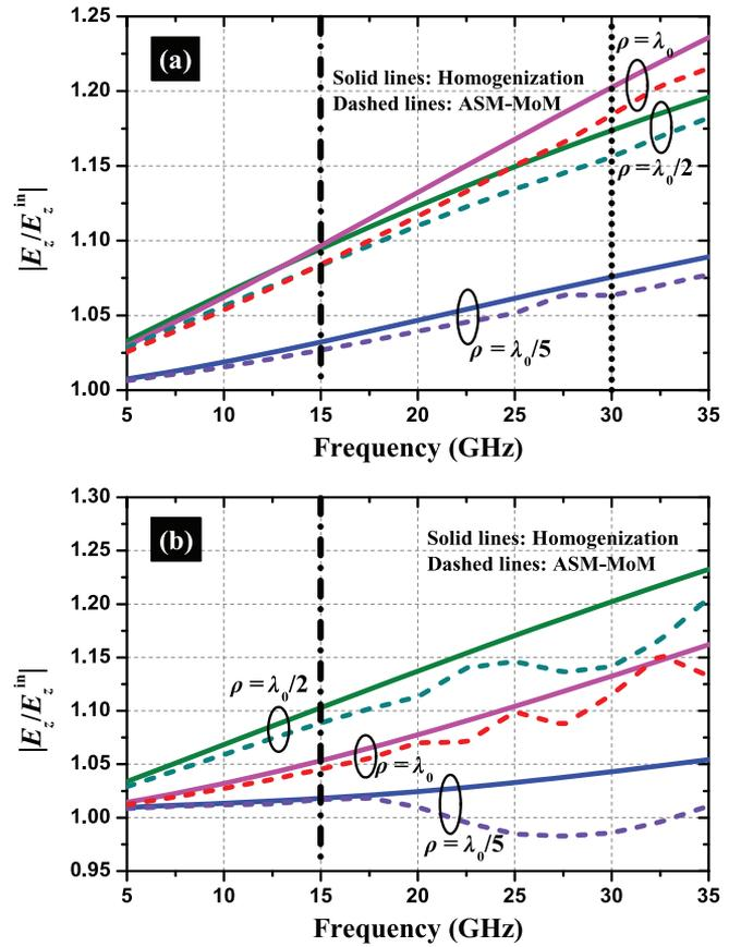
Fig. 5.  $z$ -component of electric field (normalized to the incident field) excited by a VED source above a square patch array. Parameters:  $l = 1.8$  mm,  $g = 0.2$  mm,  $x' = y' = 0$ ,  $x = y = \rho/\sqrt{2}$ . (a)  $z' = z = \lambda_0/5$  and (b)  $z' = z = \lambda_0/10$ .
