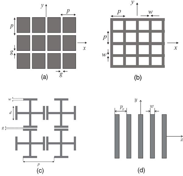
Fig. 2. (a) Square patch array. (b) Wire-mesh grid. (c) Jerusalem-cross array. (d) Strip array.
