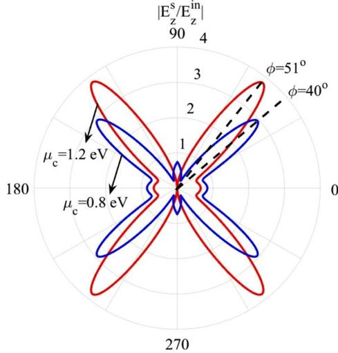
Fig. 13. Normalized scattered electric field excited by a VED source for graphene strip array with  $w = 196$  nm,  $p_x = 200$  nm, and  $f = 10$  THz. Two bias values are considered,  $\mu_c = 0.8$  eV, leading to  $\sigma_{xx} = 0.8637 + j14.2337$  mS and  $\sigma_{yy} = 0.4666 - j10.2604$  mS, and  $\mu_c = 1.2$  eV,  $\sigma_{xx} = 0.2766 + j9.8801$  mS and  $\sigma_{yy} = 0.6999 - j15.3907$  mS.
