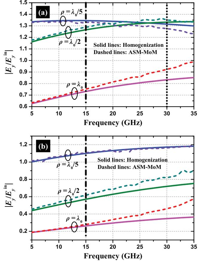
Fig. 7. Normalized  $E_y$  excited by a HED source above a wire-mesh grid. Structural parameters:  $p = 2$  mm,  $w = 0.2$  mm,  $x' = y' = 0$ ,  $x = y = \rho/\sqrt{2}$ . (a)  $z' = z = \lambda_0/5$  and (b)  $z' = z = \lambda_0/10$ .
