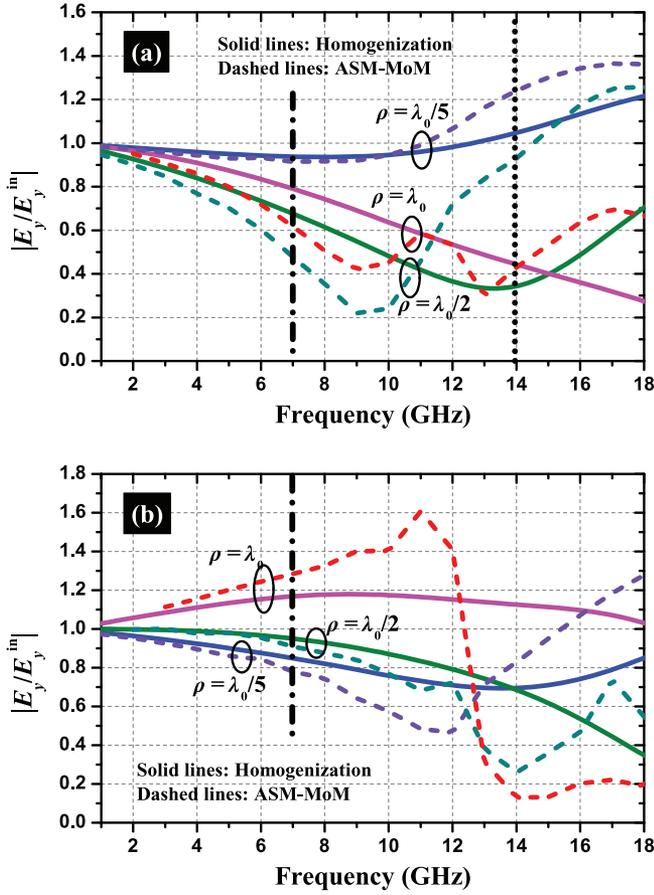
Fig. 10. Normalized  $E_y$  excited by HED source above a JC array. Structural parameters:  $p = 4.3$  mm,  $g = 0.1$  mm,  $d = 2.8$  mm,  $w = t = 0.2$  mm,  $x' = y' = 0$ ,  $x = y = \rho/\sqrt{2}$ . (a)  $z' = z = \lambda_0/5$  and (b)  $z' = z = \lambda_0/10$ .
