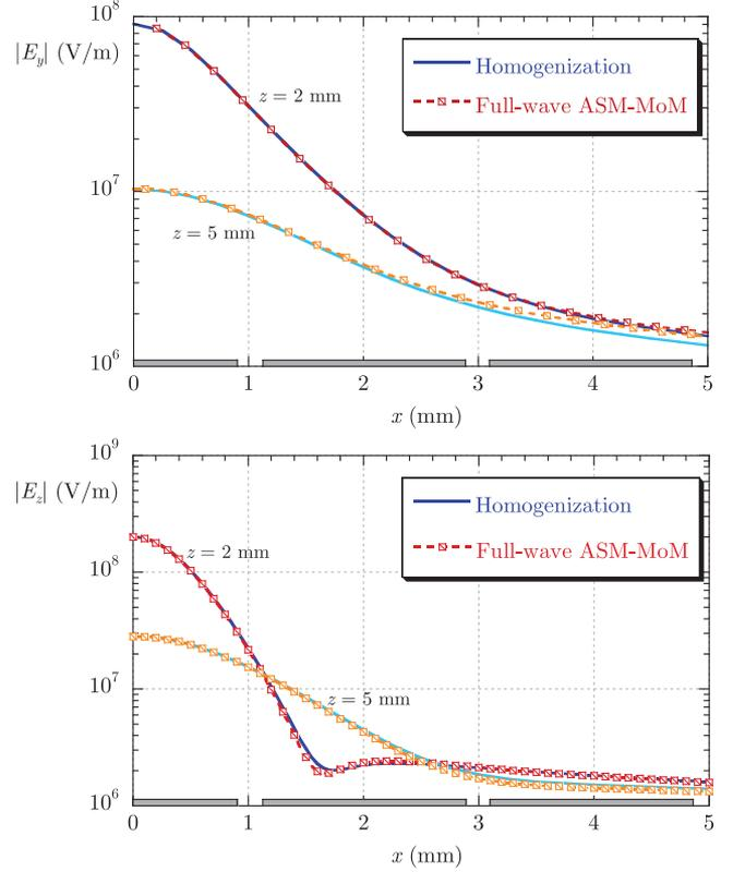
Fig. 3. Electric field excited by a 1-A HED (upper plot) or VED (lower plot) source above a square PEC patch array at  $f = 15$  GHz, for  $l = 1.8$  mm,  $g = 0.2$  mm,  $p = l + g = 2$  mm ( $p/\lambda = 0.1$ ),  $x' = 0$ ,  $y' = 0$ ,  $z' = 3$  mm, and  $y = 0$ .
