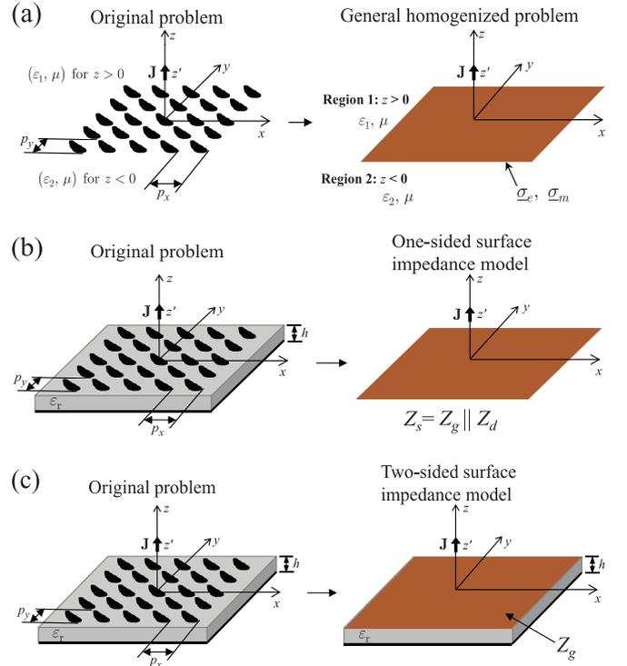
Fig. 1. Original problem and its equivalent homogenized problem represented by (a) general sheet with electric conductivity tensor  $\underline{\sigma}_e$  and magnetic conductivity tensor  $\underline{\sigma}_m$ ; (b) one-sided impedance surface; and (c) two-sided impedance surface.
