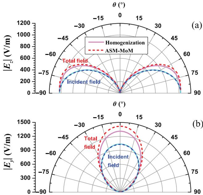
Fig. 11. Far field above a JC array (solid lines: homogenization model; dashed lines: ASM-MoM). Structural parameters:  $p = 4.3$  mm,  $g = 0.1$  mm,  $d = 2.8$  mm,  $w = t = 0.2$  mm,  $x' = y' = 0$ ,  $r = 100\lambda_0$ ,  $z = r\cos\theta$ ,  $f = 7$  GHz. (a)  $E_z$  in the  $xOz$  plane excited by a VED source,  $z' = 2p$ ,  $x = r\sin\theta$ ,  $y = 0$ . (b)  $E_y$  in the  $yOz$  plane excited by a HED source,  $z' = 3p$ ,  $x = 0$ ,  $y = r\sin\theta$ .
