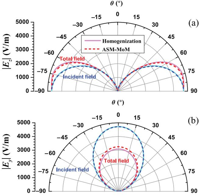
Fig. 6. Far field above a square patch array (solid lines: homogenization model; dashed lines: ASM-MoM). Structural parameters:  $l = 1.8$  mm,  $g = 0.2$  mm,  $x' = y' = 0$ ,  $r = 100\lambda_0$ ,  $z = r\cos\theta$ ,  $f = 15$  GHz. (a)  $E_z$  in the  $xOz$  plane excited by a VED source,  $z' = 3p$ ,  $x = r\sin\theta$ ,  $y = 0$ . (b)  $E_y$  in the  $yOz$  plane excited by a HED source,  $z' = p$ ,  $x = 0$ ,  $y = r\sin\theta$ .
