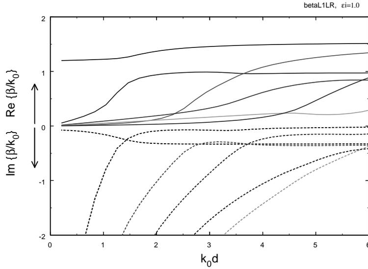
**Figure 3.** Dispersion curves for the first six  $\text{TM}^p$  modes of the two-layer waveguide shown in Fig. 1, with  $\varepsilon_3 = \varepsilon_0$ ,  $\varepsilon_2 = (2.25 - i1.0)\varepsilon_0$ , and  $d_1 = d_2 = d$  (lossy case).
