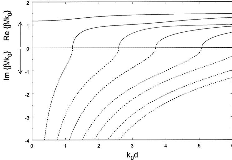
**Figure 2.** Dispersion curves for the first eight  $\text{TM}^\rho$  modes of the two-layer waveguide shown in Fig. 1, with  $\epsilon_3 = \epsilon_0$ ,  $\epsilon_2 = (2.25 - i0.0)\epsilon_0$ , and  $d_1 = d_2 = d$  (lossless case).
