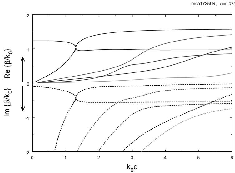
**Figure 4.** Dispersion curves for the first six  $\text{TM}^\rho$  modes of the two-layer waveguide shown in Fig. 1, with  $\varepsilon_3 = \varepsilon_0$ ,  $\varepsilon_2 = (2.25 - i1.735523)\varepsilon_0$ , and  $d_1 = d_2 = d$  (first two modes are degenerate).
