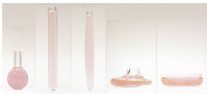
Fig. 4. Container shapes containing solutions. Left to right: sphere (1 mL), tube (0.65 mL), prolate spheroid (0.7 mL), oblate spheroid (1 mL), dish (1 mL).
