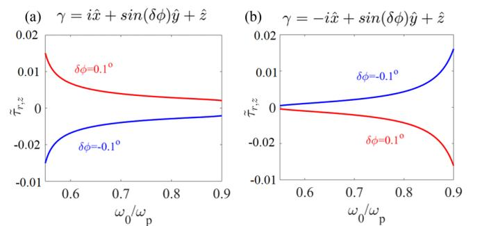
FIG. 6. Normalized optical torque  $\tau_z$ , in the frequency range  $[\omega_-, \omega_+]$ , exerted on an LCP atom (a) and an RCP atom (b), with the polarization plane tilted from the  $xoz$  plane by a small angle  $\delta\phi$ . The torque tends to align the polarization plane of an LCP atom to the  $xoz$  plane, whereas it tends to rotate the polarization plane of an RCP atom out of the  $xoz$  plane.
