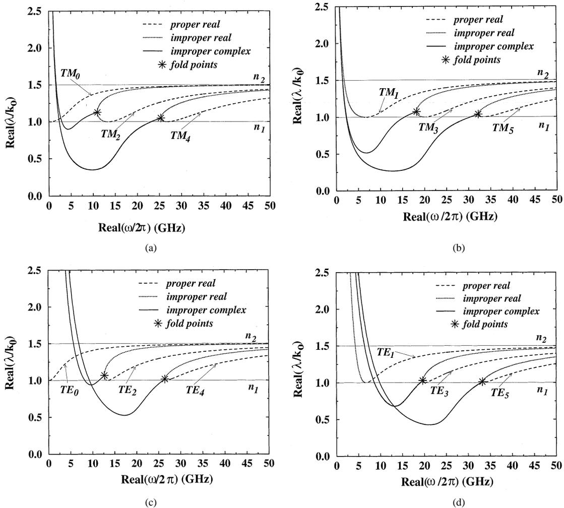
Fig. 3. Dispersion curves of bound and leaky modes for an isotropic planar waveguide having  $\epsilon \equiv \epsilon_2 = 2.25\epsilon_0$ ,  $\epsilon_1 = \epsilon_0$ , and  $2d = 2$  cm. (a)  $TM^p$ -even modes. (b)  $TM^p$ -odd modes. (c)  $TE^p$ -even modes. (d)  $TE^p$ -odd modes. A star symbol denotes the fold singular point associated with the leaky-wave cutoff.
