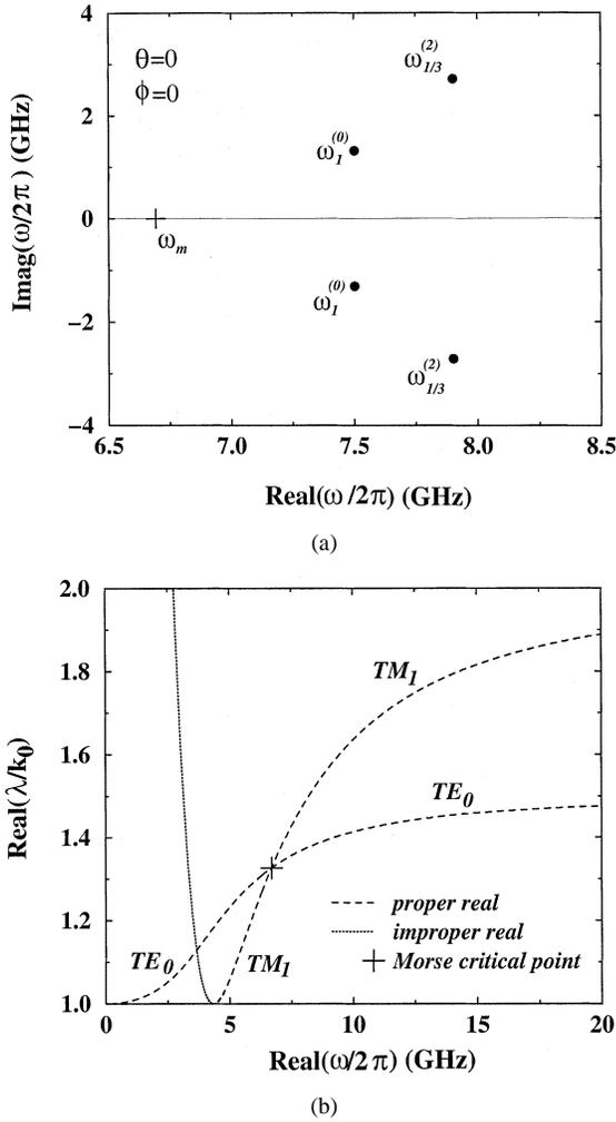
Fig. 5. (a) Complex frequency-plane singularities associated with the first two modes shown in Fig. 2. The optical axis is positioned at  $\theta = 0^\circ$  (pure uncoupled  $TE^p$  and  $TM^p$  modes exist). (b) Dispersion curves for the first two modes shown in Fig. 2 when the optical axis is positioned at  $\theta = 0^\circ$ . The location of a degenerate MCP given by (12) is shown by the plus sign at the place of intersection of dispersion curves.
