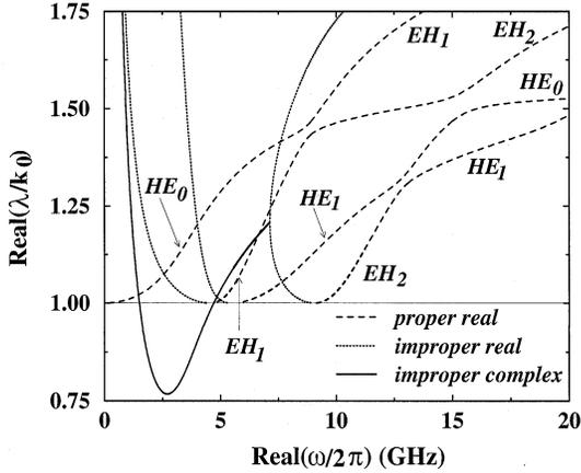
Fig. 2. Dispersion curves for the first four modes of an anisotropic planar waveguide having permittivity (2), where  $\epsilon_{xx} = \epsilon_{yy} = 4\epsilon_0$ ,  $\epsilon_{zz} = 2.25\epsilon_0$ , and  $2d = 2$  cm. The optical axis is positioned at  $\theta = 45^\circ$  and  $\phi = 30^\circ$ . The modes are hybrid, and couple together due to the asymmetry provided by the placement of the optical axis.
