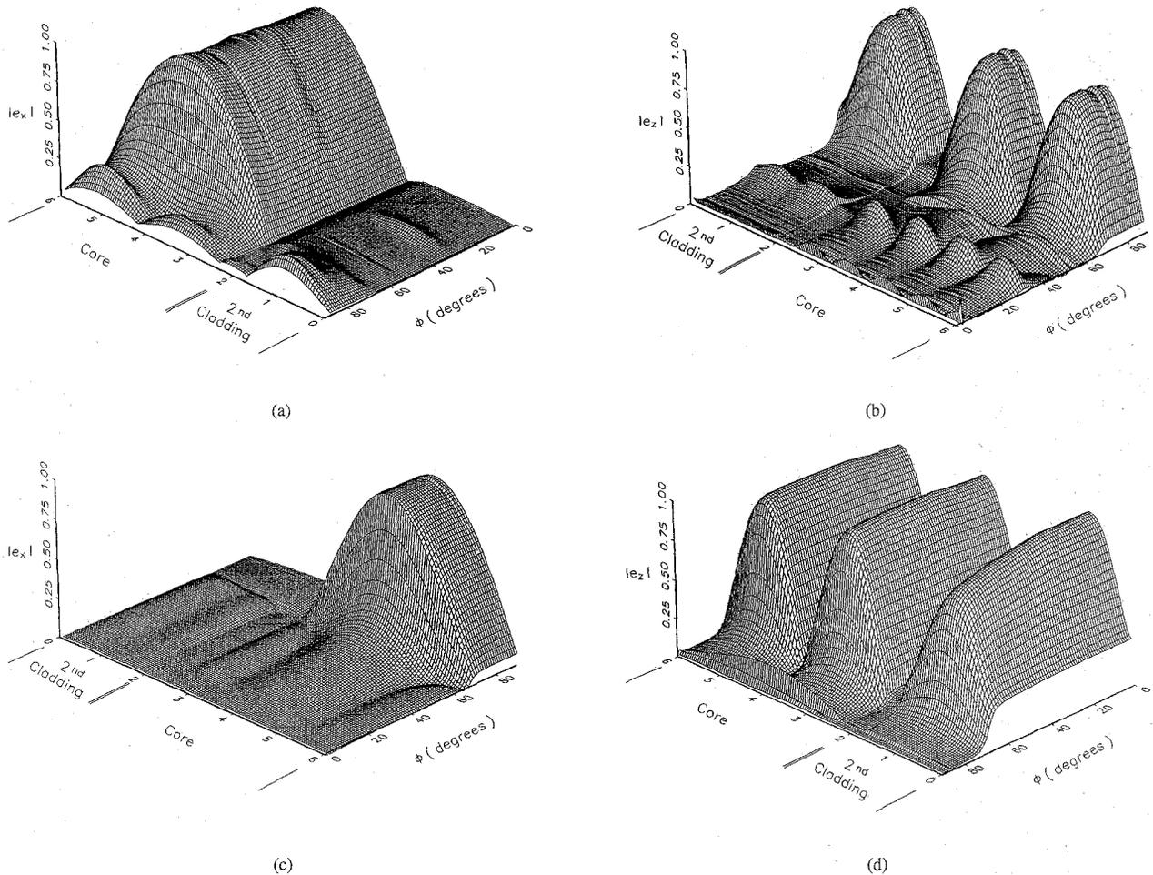
Fig. 5. Field component  $e_x$  (a) and  $e_z$  (b) versus position and rotation angle in the polar plane for  $TE_0 \rightarrow TM_0$  mode evolution as  $\phi = 0^\circ \rightarrow 90^\circ$ ,  $\theta = 0^\circ$ ,  $AR = 1.03$ . Field component  $e_z$  (c) and  $e_x$  (d) versus position and rotation angle in the polar plane for  $TM_1 \rightarrow TE_0$  mode evolution as  $\phi = 0^\circ \rightarrow 90^\circ$ ,  $\theta = 0^\circ$ ,  $AR = 1.03$ .
