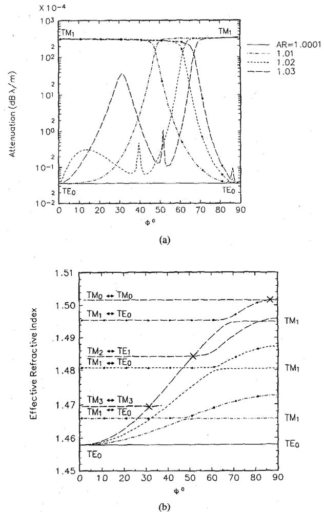
Fig. 4. Attenuation (a) and effective refractive index (b) versus orientation of optic axis in polar ( $x$ - $y$ ) plane for various values of AR. Mode evolution  $TE_0 \rightarrow TM_1$  (no dots) and  $TM_1 \rightarrow TE_0$  (dots) occurs with increasing angle  $\phi$ ,  $\theta = 90^\circ$ .
