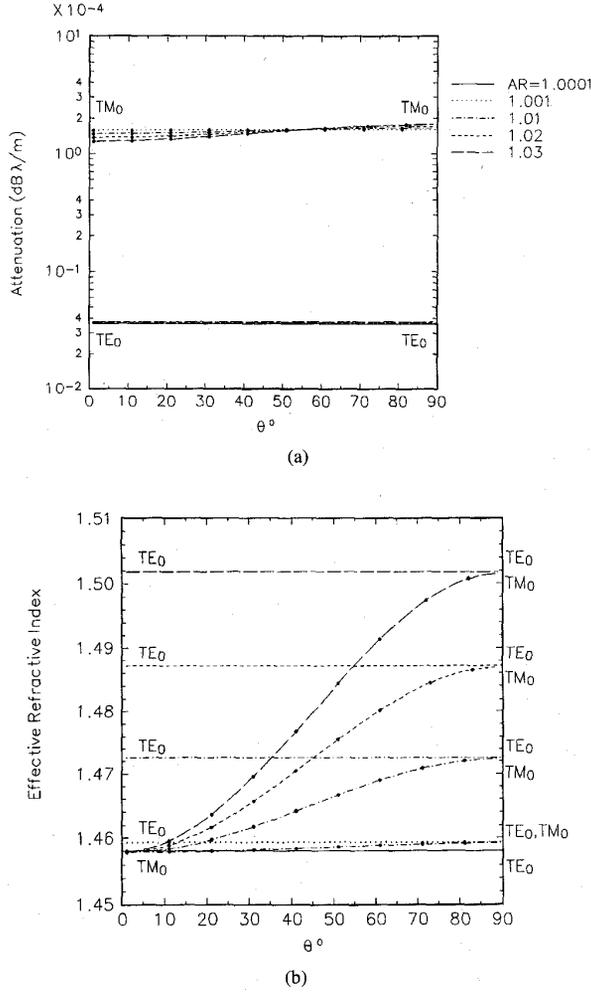
Fig. 6. Attenuation (a) and effective refractive index (b) versus orientation of optic axis in the equatorial  $z$ - $y$  plane for various values of AR. Pure  $TE_0$  (no dots) and  $TM_1$  (dots) modes exist for all angles of rotation  $\theta$ ,  $\phi = 90^\circ$ .
