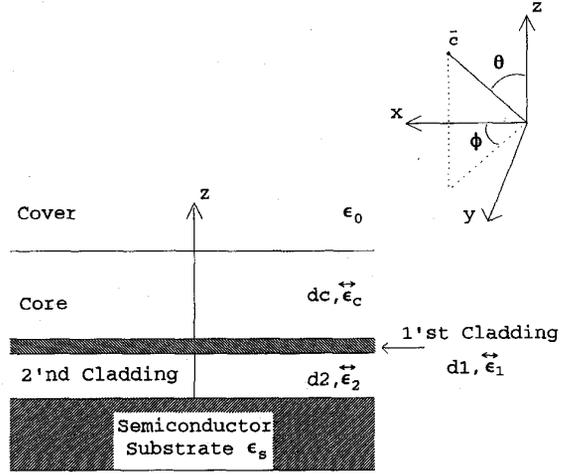
Fig. 1. Anisotropic ARROW waveguiding structure.
