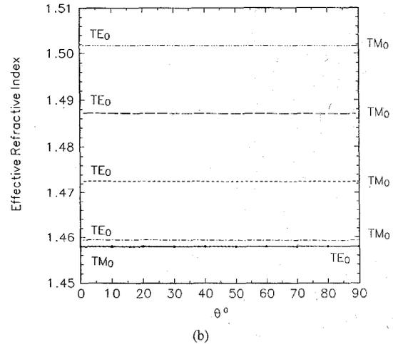
Fig. 2. Attenuation (a) and effective refractive index (b) versus orientation of optic axis in transverse ( $z$ - $x$ ) plane for various values of AR. Mode evolution  $TE_0 \rightarrow TM_0$  (no dots) and  $TM_0 \rightarrow TE_0$  (dots) occurs with increasing angle  $\theta$ ,  $\phi = 0^\circ$ .
