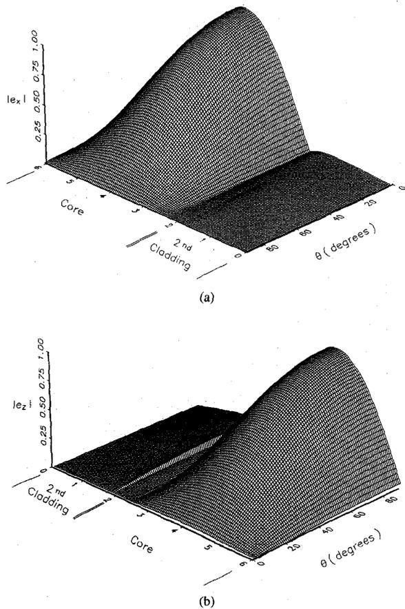
Fig. 3. Field component  $e_x$  (a) and  $e_z$  (b) versus position and rotation angle in the traverse plane for  $TE_0 \rightarrow TM_0$  mode evolution as  $\theta = 0^\circ \rightarrow 90^\circ$ ,  $\phi = 0^\circ$ ,  $AR=1.03$ .
