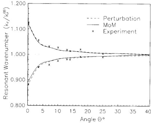
Fig. 5. Comparison of perturbation-theory-predicted, MoM predicted, and experimentally measured system wavenumbers for two identical coupled microstrip disks as the angle between them is varied.  $\epsilon_f = 2.20$ ,  $t = .0787$  cm,  $l = 2.5$  cm,  $w = .0784$  cm,  $d_1 = 0.1$  cm,  $d_2 = 2.6$  cm
