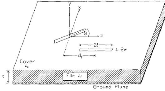
Fig. 1. Configuration of two identical coupled microstrip disks.
