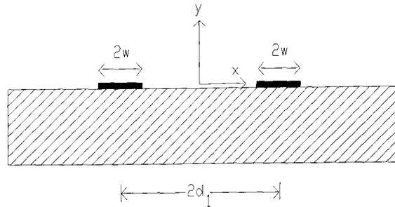
Fig. 2. Two coupled disks with transverse separation  $2d_1$ .
